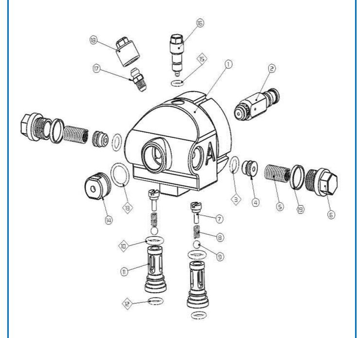
Note: Use the parts breakdown for the "**MULTI SPRAY 5**" Head Assembly as a guide for servicing and repairing the unit.
